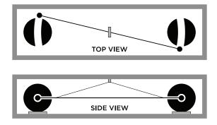
Fig. 1. – Schematic of modified Cavendish balance. Since the idea is to demonstrate the simple harmonic motion only as a first approximation, deviation due to the slight arc in the trajectory is inconsequential.
